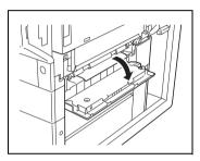
2 Turn the green wheels to feed the paper so that it can be easily removed.
